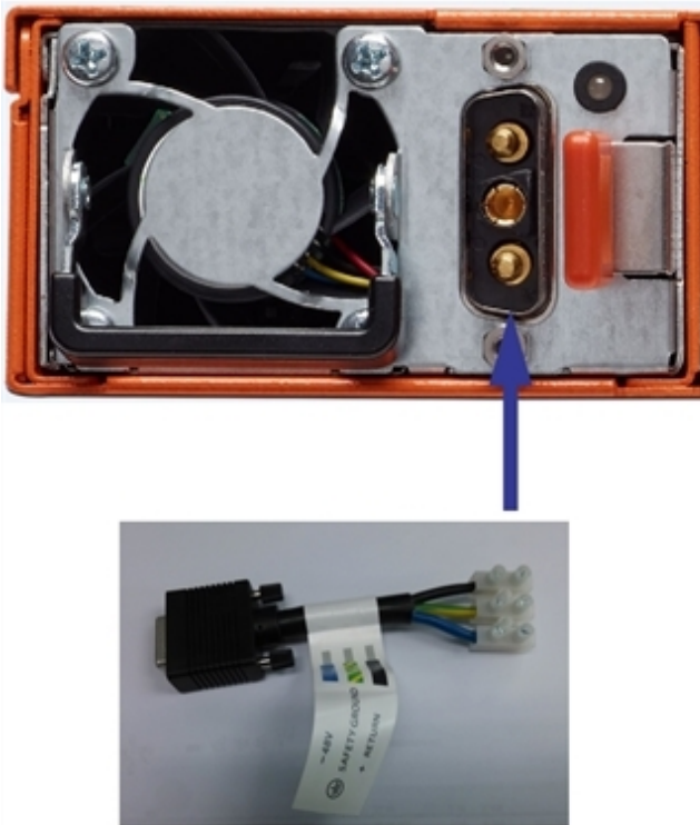
Figure 4: DC Power Module
