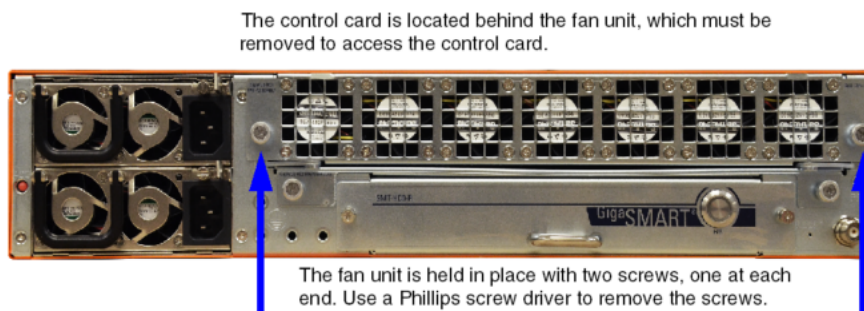
Figure 1: Replacing a Control Card
